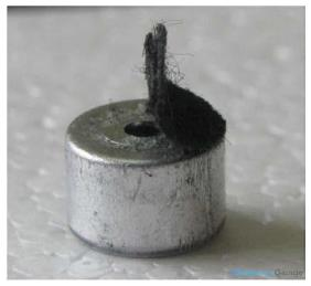
A solid conducting metal body encapsulates the various parts of the microphone. The top face is covered with a porous material with the help of glue. It acts as a filter for the dust particles. The sound signals/air vibrations passes through the porous material and falls on the diaphragm through the hole shown in the image above.
