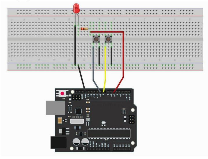
Although the bodies of the switches are square, the pins protrude from opposite sides of the switch. This means that the pins will only be far enough apart when they are placed correctly on the breadboard.
