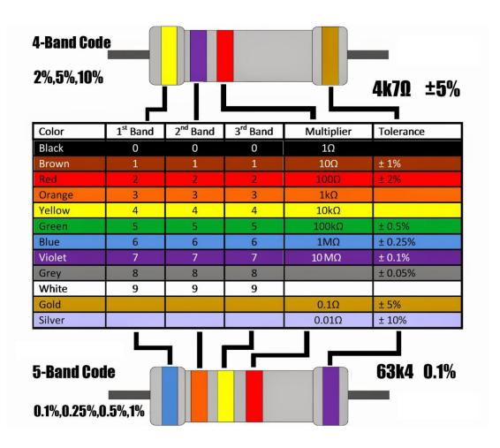
Unlike LEDs, resistors do not have a positive and negative lead. They can be connected either way around.
