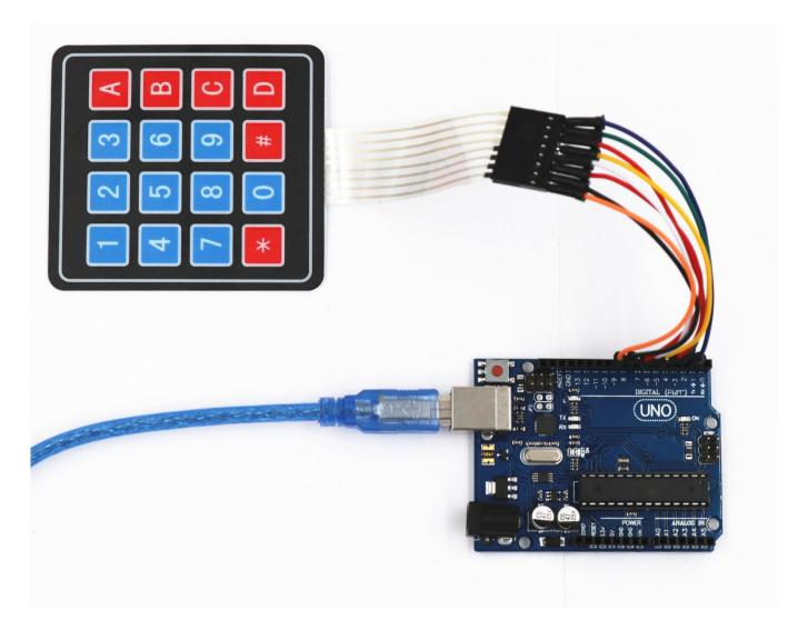
With this code, once we press a key on the keypad, it should show up on the serial monitor of the Arduino software once the code is compiled and uploaded to the UNO R3 board.
