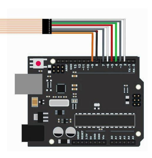
When connecting the pins to the UNO R3 board, we connect them to the digital output pins, D9-D2. We connect the first pin of the keypad to D9, the second pin to D8, the third pin to D7, the fourth pin to D6, the fifth pin to D5, the sixth pin to D4, the seventh pin to D3, and the eighth pin to D2.
