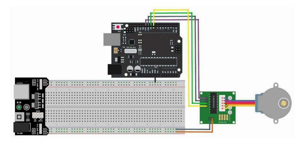
We are using 4 pins to control the Stepper. Pin 8-11 are controlling the Stepper motor. We connect the Ground from to UNO to the Stepper motor.
