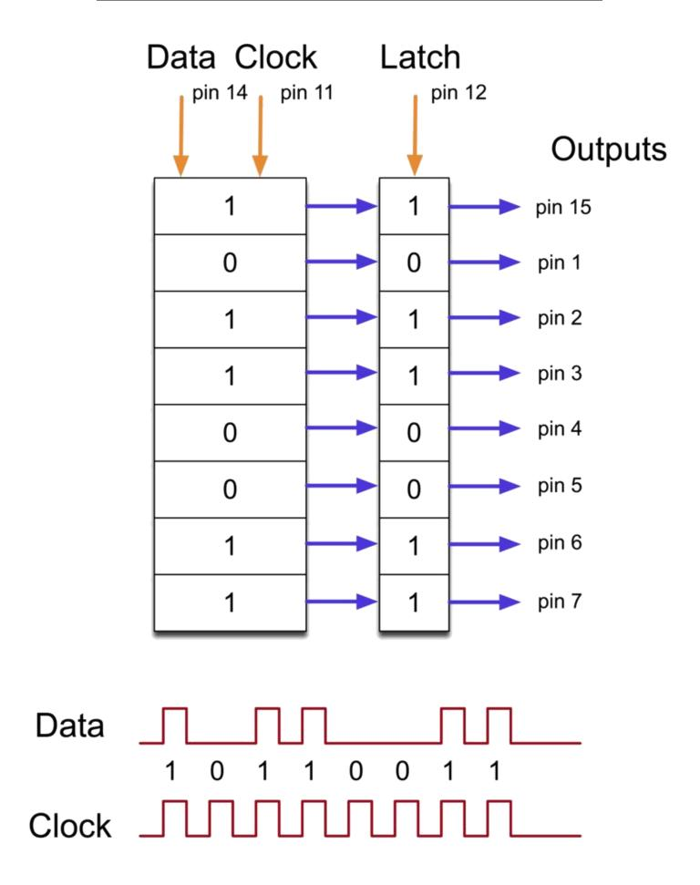
The clock pin needs to receive eight pulses. At each pulse, if the data pin is high, then a 1 gets pushed into the shift register; otherwise, a 0. When all eight pulses have been received, enabling the 'Latch' pin copies those eight values to the latch register. This is necessary; otherwise, the wrong LEDs would flicker as the data is being loaded into the shift register.
