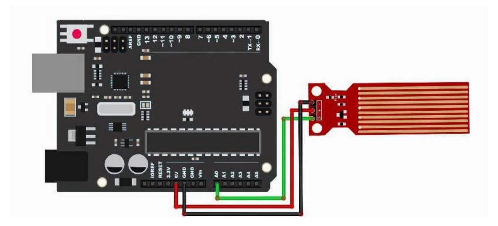
Wiring tips: Power supply (+) is connected to 5V of UNO R3 board, ground electrode (-) is connected to GND. Signal output (S) is connected to the ports (A0-A5) which have function of inputting analog signal in UNO R3 board, random one is OK, but it should define the same demo code as the routine.
