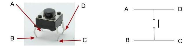
Actually, there are only really two electrical connections. Inside the switch package, pins B and C are connected together, as are A and D.
