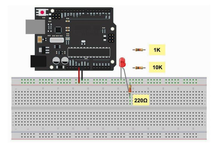
The UNO is a convenient source of 5 volts, which we will use to provide power to the LED and the resistor. You do not need to do anything with your UNO, except to plug it into a USB cable.
