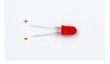
If you do not use a resistor with an LED, then it may well be destroyed almost immediately, as too much current will flow through, heating it and destroying the 'junction' where the light is produced.
