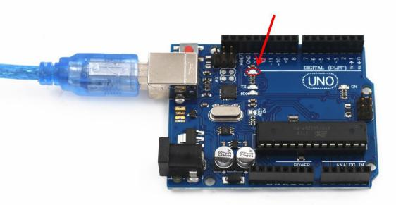
You may find that your UNO R3 board's 'L' LED already blinks when you connect it to a USB plug. This is because the boards are generally shipped with the 'Blink' sketch pre-installed.
