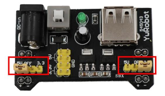
The left and right voltage output can be configured independently. To select the output voltage, move jumper to the corresponding pins. Note: power indicator LED and the breadboard power rails will not power on if both jumpers are in the "OFF" position.
