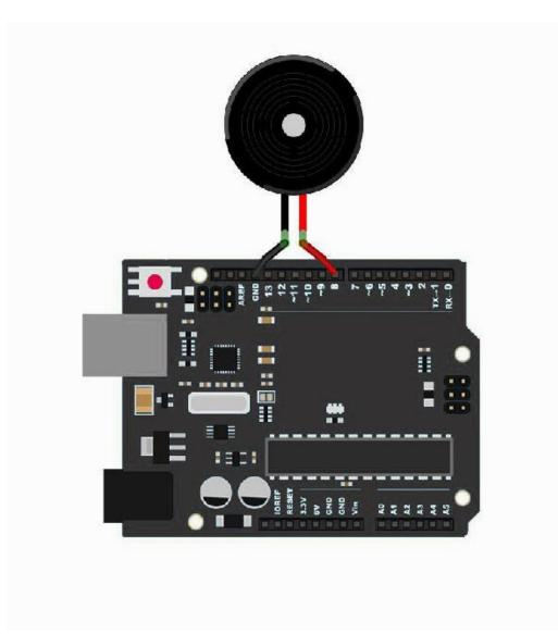
Wiring the buzzer connected to the UNO R3 board, the red (positive) to the pin8, black wire (negative) to the GND.
