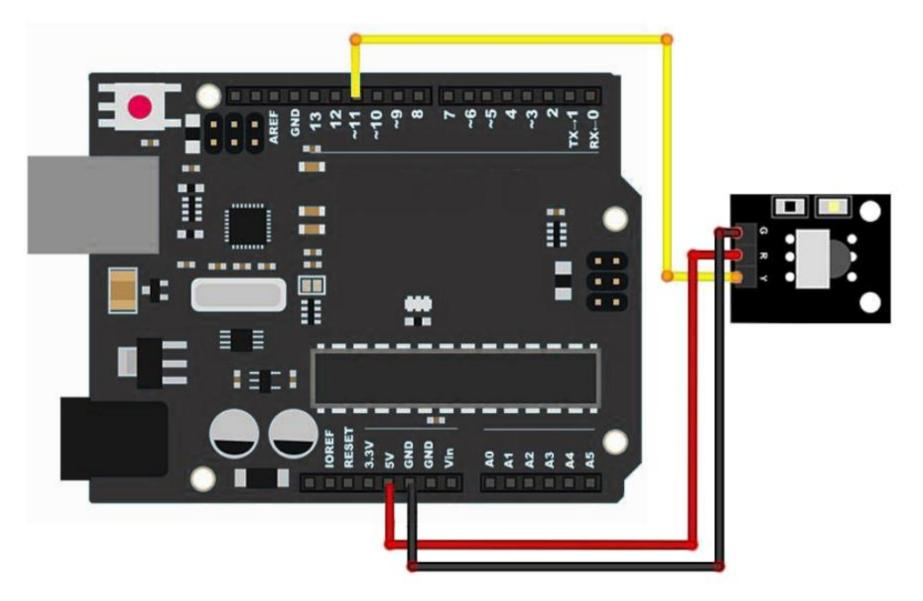
There are 3 connections to the IR Receiver. The connections are: Signal, Voltage and Ground. The "-" is the Ground, "S" is signal, and middle pin is Voltage 5V.
