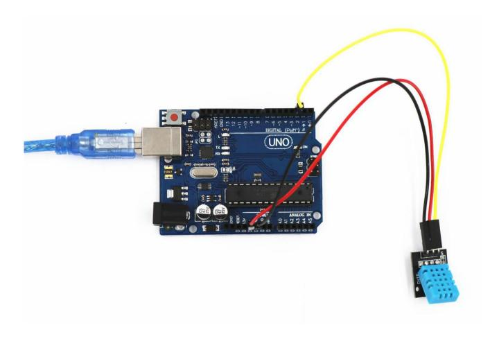
Upload the program then open the monitor, we can see the data as below: (It shows the temperature of the environment, we can see it is 22 degree)
