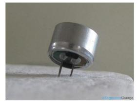
These microphones are widely used in electronic circuits to detect minor sounds or air vibrations which in turn are converted to electrical signals for further use. The two legs as shown in the image above are used to make electrical connection with the circuit.
