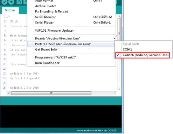
Note: The Board Type and Serial Port here are not necessarily the same as shown in picture. If you are using 2560, then you will have to choose Mega 2560 as the Board Type, other choices can be made in the same manner. And the Serial Port displayed for everyone is different, despite COM 26 chosen here, it could be COM3 or COM4 on your computer. A right COM port is supposed to be COMX (arduino XXX), which is by the certification criteria.
