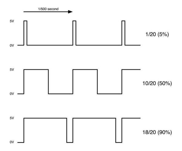
Roughly every 1/500 of a second, the PWM output will produce a pulse. The length of this pulse is controlled by the 'analogWrite' function. So 'analogWrite(0)' will not produce any pulse at all and 'analogWrite(255)' will produce a pulse that lasts all the way until the next pulse is due, so that the output is actually on all the time.
