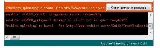
It can mean that your board is not connected at all, or the drivers have not been installed (if necessary) or that the wrong serial port is selected.
