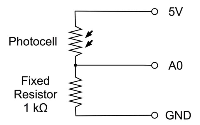
The resistor and photocell together behave like a pot. When the light is very bright, then the resistance of the photocell is very low compared with the fixed value resistor, and so it is as if the pot were turned to maximum.
